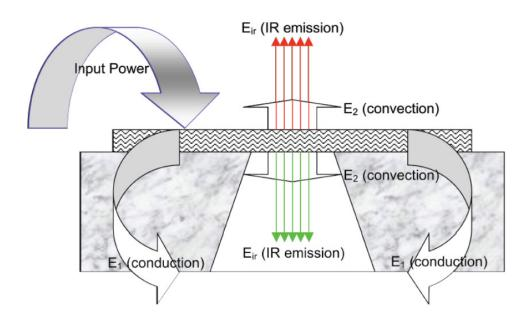
The power E<sub>0</sub>, input electrically, is dissipated by the Emitter in three ways,
